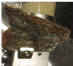
Figure 1. A mineral sample mounted on the sample holder in the reaction chamber.
