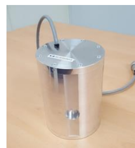
Figure 2. Large prototype of irradiator to test mechanics of a moving lead shield and electronics.
