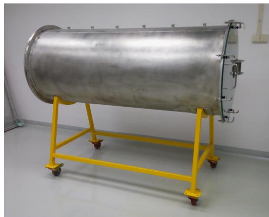
Figure 1. Cylinder chamber for ^{222}\text{Rn} measurements.
