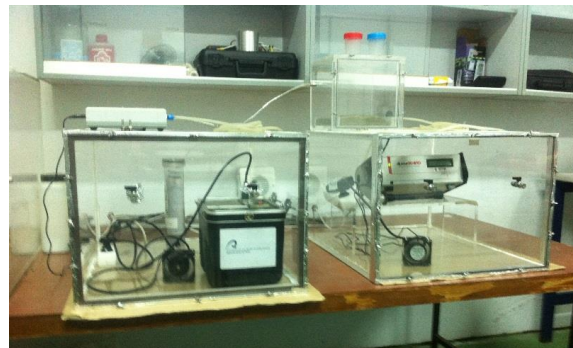
Figure 1. Radon Accumulation chamber
